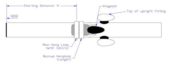
The hang loop is attached around the keel and should be within the following range. A recommended starting position is also shown. (If for example the hang loop had been removed and you are not sure where to replace it.) When you get the best position for yourself, mark the keel with a 'felt' tip pen or record a measurement for future reference. (Do not use pencil or any other implement to mark the glider.)
