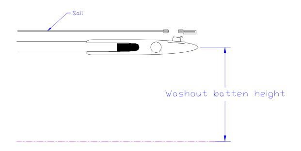
By walking behind the glider all the measurements can be recorded and written down (make sure the keel is central):
