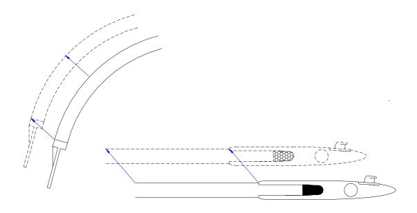
Move the batten over the profile as shown above
