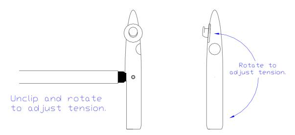
The Rio 2 battens are similar in design to those used in the high performance Cheetah and Evo competition gliders from Avian. The snap fitting allows neat robust fitting, easy rigging and easy precise adjustment of batten tension. The batten tension does make a difference to how the glider flies and is therefore important. The tension can be adjusted by rotating the clip end when open. One turn alters the tension by 1mm.
